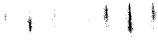
Fig. 3. RHEED streaks acquired on as-deposited (left) and after annealing at 250 °C (right) 8-Å-thick Co layers. Before annealing streaks are blurred, but single and correspond to the lattice constant 2.72 Å. After annealing they are split revealing the lattice parameter 2.59 Å and 2.83 Å for outer and inner, respectively.
