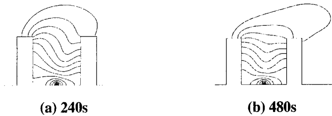
Figure 7 The iso-contours of concentration for B/H=1 by LES
