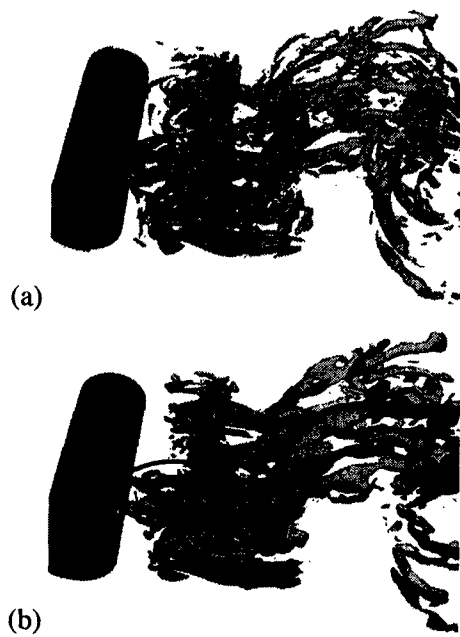
Figure 5. 3-D type shear-layer vortices and streamwise vortices: (a) iso-surface of \lambda_2 = -10 ; (b) iso-surfaces of \omega_x = +10 (light color) and \omega_x = -10 (dark color).
