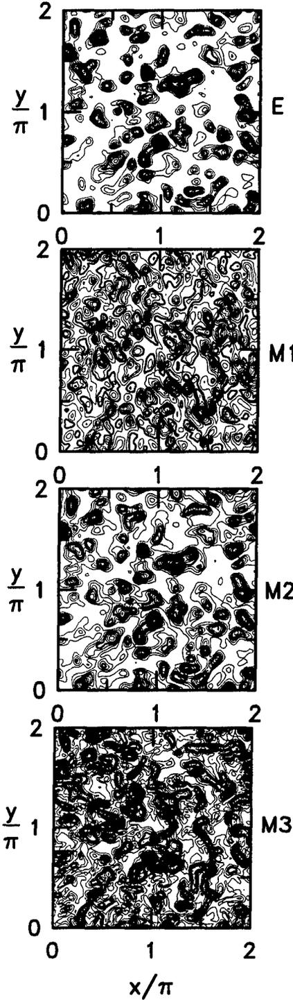
Figure 4. Planar contours of exact (*E*) and modeled (*M1*-Smagorinsky, *M2*-similarity, *M3*-gradient) SGS stresses ( $\tau_{11}$  component).
