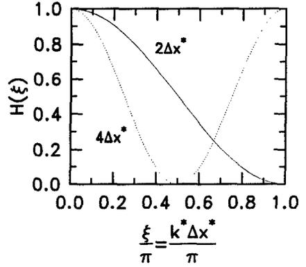
Figure 5. Transfer functions of three-point top-hat filters.
