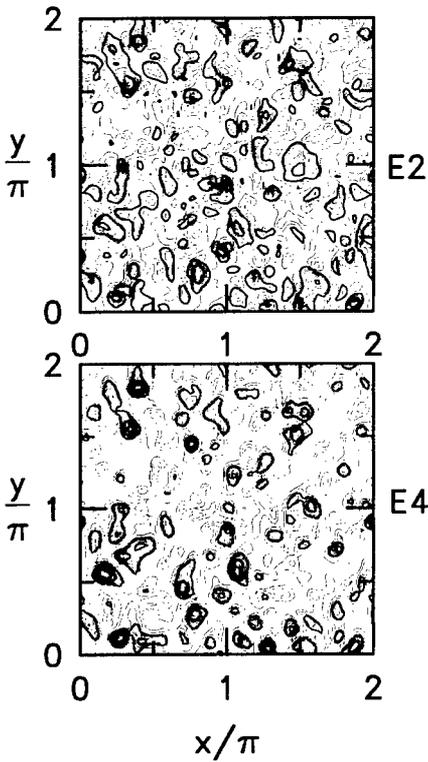
Figure 2. Exact SGS stresses from grid filters of 2nd- (E2) and 4th-order (E4).
