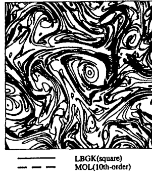
Figure 8. Comparison of vorticity contours between LBGK(square) and MOL(10th-order) at t = 3.0 , \nu = 0.0001
