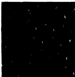
Figure 1. Tapping mode AFM image of the Ag nanoparticle LSPR nanosensor. After solvent annealing, the resulting nanoparticles have in plane widths of \sim 100 nm and out-of-plane heights of 51 nm. Defects are present in sensing probe volume but do not contribute to the optical sensing events.
