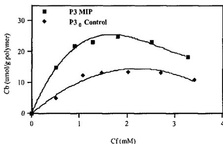
**Figure 3.** The rebinding of dAMP **11** to MIP **P3** is compared to its rebinding with non-imprinted polymer **P3<sub>0</sub>**. (**P3** was imprinted for adenosine dimer **1**).
