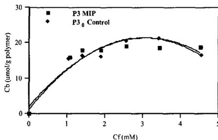
**Figure 4.** The rebinding of dGMP **12** to MIP **P3** is compared to its rebinding with non-imprinted polymer **P3<sub>0</sub>**. (**P3** was imprinted for adenosine dimer **1**).
