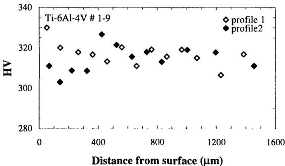
Figure 5 Vickers microhardness profiles on a Ti-6Al-4V specimen.
