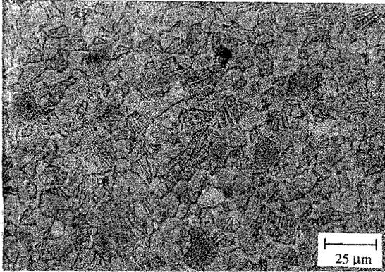
Figure 1 Microstructure of the heat-treated titanium alloy consisting of  $\alpha$  and transformed  $\beta$  in an acicular structure, with an  $\alpha$  grain size of  $\sim 7.5 \mu\text{m}$ . (500 X)
