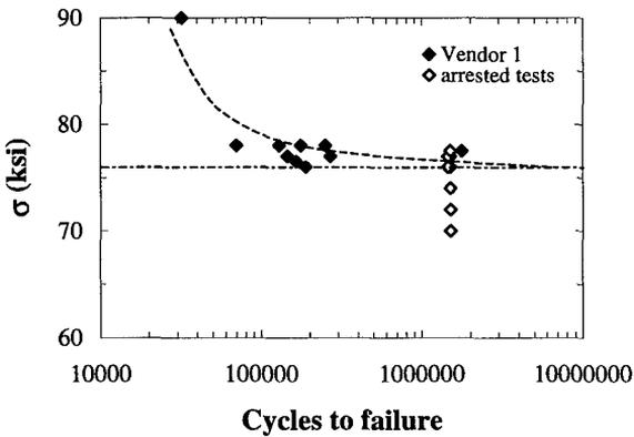
Figure 2 S-N curve for specimens shot peened by Vendor 1 with an endurance limit of  $\sim 76$  ksi.
