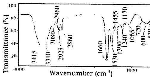
**Fig. 8.** Characteristic IR bands of artificial cobweb
