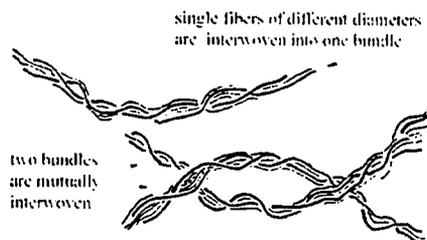
**Fig. 1.** Simplified drawing of artificial cobweb (yarn)
