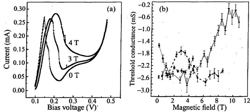
**Fig. 2.** (a) Current–voltage characteristics of the RTD at different in-plane magnetic fields. (b) Threshold conductance versus in-plane magnetic field. Circles with dotted line correspond to data measured on sample A. Squares with dash line correspond to sample B. Triangles with solid line correspond to sample C. Lines is used only as viewguide.
