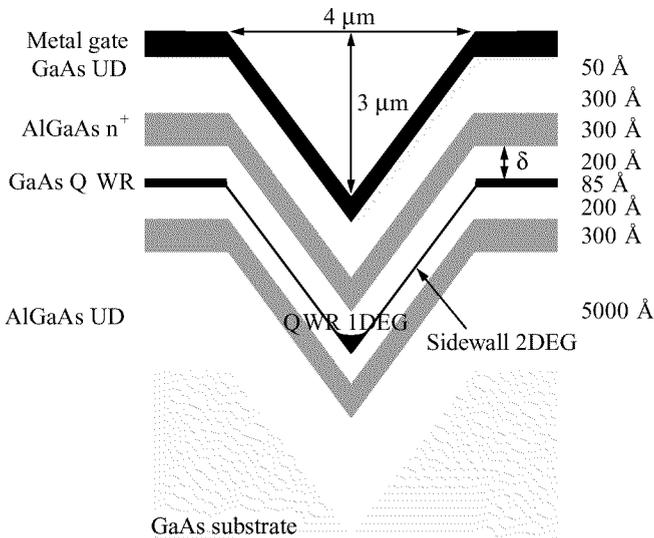
Fig. 1. Schematic cross-sectional picture of a QWR heterostructure.
