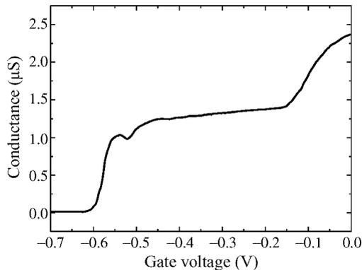
Fig. 4. Conductance vs gate voltage at 4.2 K.
