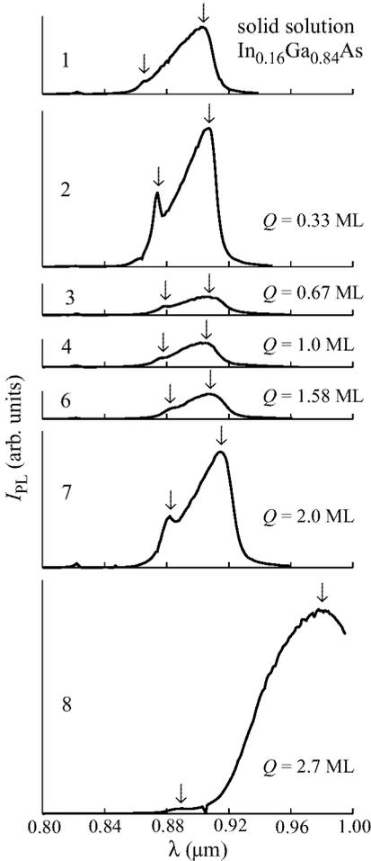
**Fig. 1.** Photoluminescence spectra of modulation doped InAs/GaAs superlattices with InAs layer thickness  $Q$  from 0.33 up to 2.7 monolayer and the mean composition  $\text{In}_{0.16}\text{Ga}_{0.84}\text{As}$  sample.
