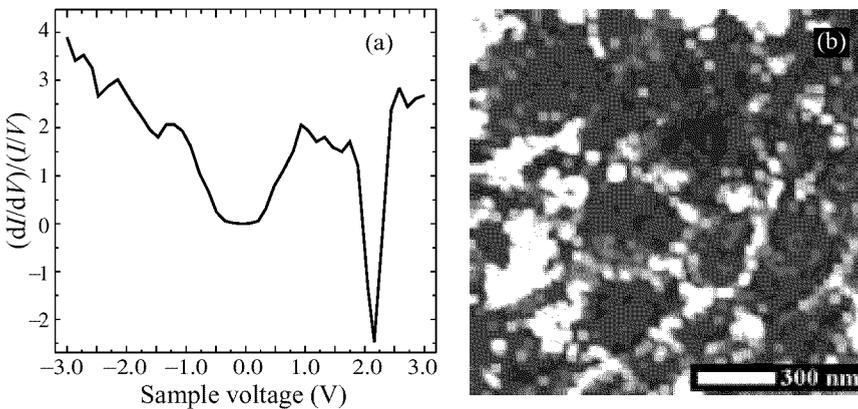
**Fig. 2.** (a) The  $(dI/dV)/(I/V)$  curve, showing negative differential conductance at about +2.2 V sample voltage, recorded at the contact region of two spheres of a sample. (b) CITS image acquired at -1.75 V sample voltage in one of the opals. Gray scale range is 2.9 nA.
