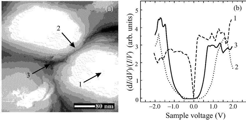
**Fig. 1.** (a) Constant current STM image showing the contact region of three spheres of an opal. (b) The  $(dI/dV)/(I/V)$  spectra recorded at regions marked in Fig. 1(a). Curves 1 and 2 are usually obtained at regions marked as 1 in the image. Curve 3 is usually recorded at regions labeled 2 in the figure. Spectra obtained at regions labeled as 3 are similar to curve 1.
