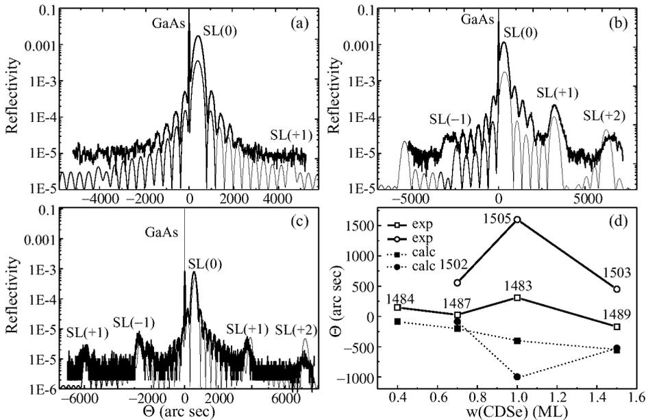
**Fig. 1.** Experimental (thick line) and simulated (thin line) DCD (002) rocking curves for (a) CdTe/BeTe SL (#1480); (b) CdSe/BeTe SL with the max-max CdTe interfaces (#1483); (c) CdSe/BeTe SL with the min-max CdTe interfaces (#1502). Angular position of the SL(0) peak at 002-rocking curves for the samples of the first set (squares) and the second set (circles) as a function of CdSe nominal thickness is presented in (d).
