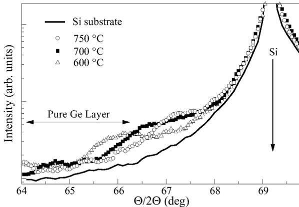
**Fig. 2.** The  $\Theta/2\Theta$  X-ray scans of samples grown at different temperature near (004) Si reflection. The arrows mark angle region of diffraction from pure Ge layer at different strain and peak position from Si substrate.
