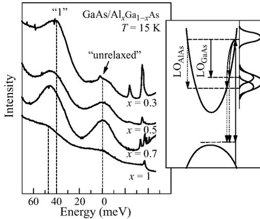
**Fig. 3.** Hot electron luminescence spectra for four GaAs/Al<sub>x</sub>Ga<sub>1-x</sub>As multiple quantum wells samples plotted as a function of the electron energy above the ground state of the quantum wells. The inset shows schematically the principles of the hot electron neutral acceptor luminescence technique.
