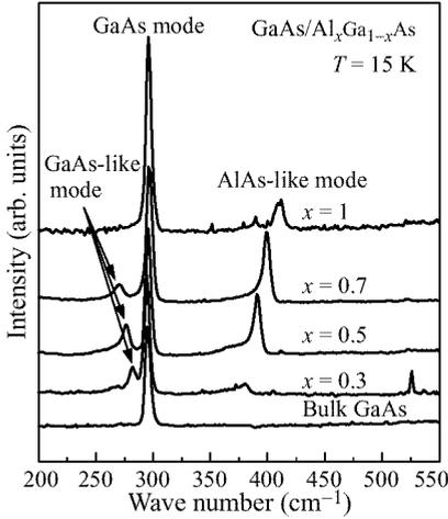
**Fig. 1.** Raman spectra of four GaAs/ $\text{Al}_x\text{Ga}_{1-x}\text{As}$  multiple quantum wells and bulk GaAs samples at 15 K in the back scattering geometry for incident wavelength of 514.5 nm. The peak labeled GaAs mode is the LO phonon arising from the GaAs wells. The other two peak labeled GaAs like and AlAs-like mode are related to the  $\text{Al}_x\text{Ga}_{1-x}\text{As}$  barrier layers.
