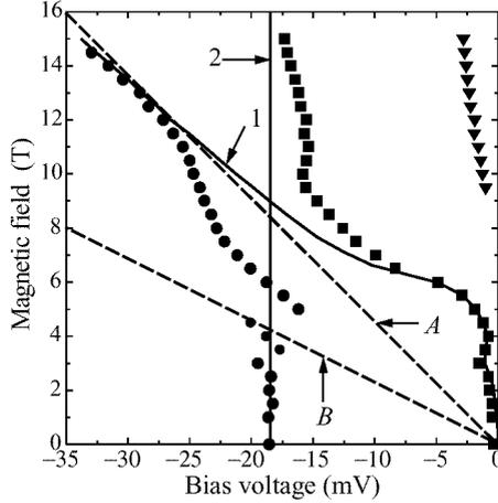
**Fig. 2.** Peak positions on the voltage scale as a function of magnetic field. Circles, squares and triangles represent experimental data and are discussed in the text. Curves “1” and “2” represent expected peak position calculated in the absence of the interactions between Landau levels. Lines “A” and “B” represent tunneling between Landau levels with  $\Delta N = 1$  and  $\Delta N = 2$  correspondingly in the case of the ideal Landau level quantization.
