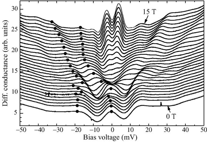
**Fig. 1.** Tunneling differential conductance at 4.2 K as a function of external voltage in different magnetic fields. The curves are shifted for clarity in vertical direction. The lowest curve is for  $B = 0$  T, the top one — for  $B = 15$  T. Magnetic field step between curves  $\Delta B = 0.5$  T. The curve for  $B = 0.5$  T is absent. Circles mark the peaks which evolution with magnetic field are discussed in the paper.
