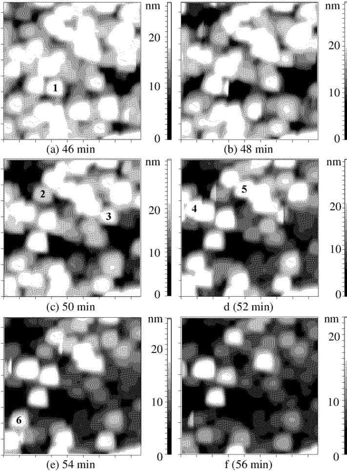
**Fig. 1.** The series of the AFM images shows the transformation of the same area ( $860 \times 860$  nm) of  $\text{SiO}_2$  with  $\alpha\text{Fe}$  nanoparticles during the chemical etching, when the tip apex are pushing out some of the protrusions corresponding to the nanoparticles (with numbers 1–6). In brackets there was indicated the time from start of the chemical etching process.
