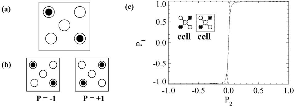
**Fig 1.** (a) A quantum-dot cell consisting of five dots is occupied by two electrons. (b) The two distinct ground-state configurations with their polarizations. (c) Cell-cell coupling characteristics.
