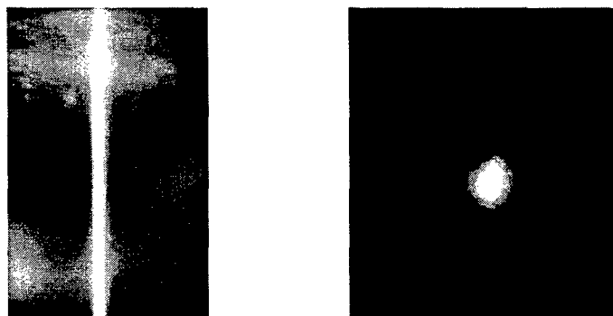
Figure 6 photograph of the liquid Xenon jet (left) and of the laser plasma generated on the jet (right)
