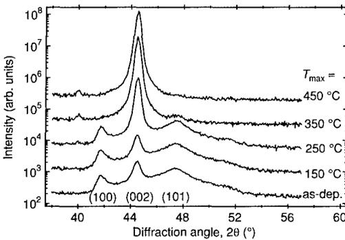
**Figure 4.** Reflections of hcp-Co as measured by XRD for the as-deposited and annealed Co films (annealing temperature  $T_{\max}$ , as indicated). The increasing abundance of c-axis texture component is indicated by the intensity changes of the reflections.
