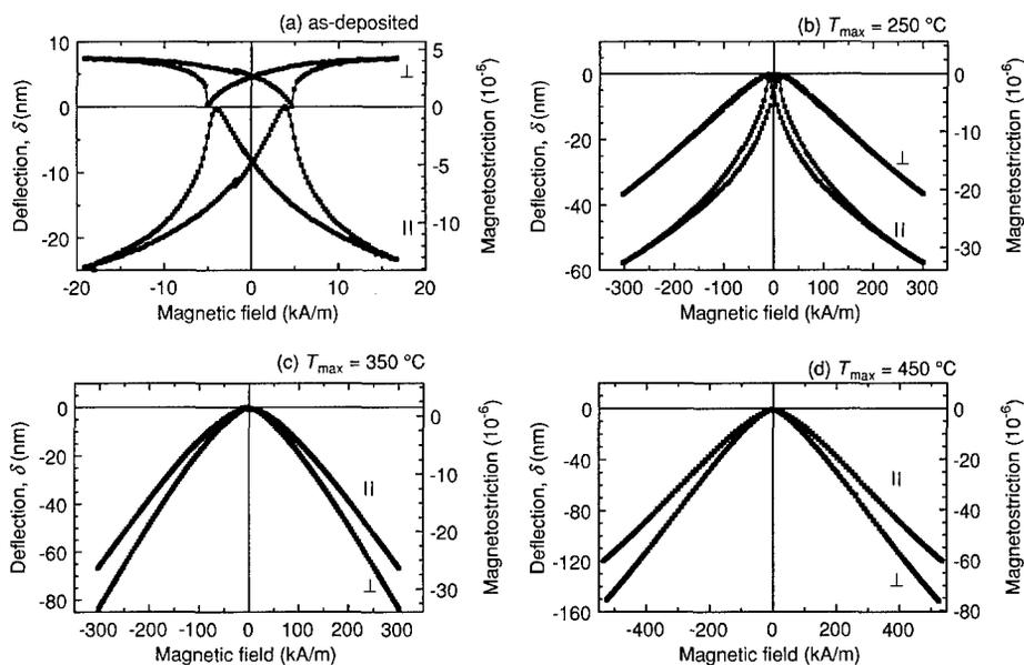
**Figure 2.** Magnetostrictive deflection and magnetostriction in longitudinal ( $\parallel$ ) and transverse ( $\perp$ ) magnetic fields during the second magnetization loop. The behavior changes strongly during annealing at  $T_{\max} \geq 250$  °C.
