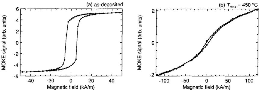
**Figure 5.** MOKE signals of the as-deposited and an annealed ( $450\text{ }^{\circ}\text{C}$ ) Co film demonstrate the surface magnetization behavior. Main features correspond to the deflection changes in figure 2.
