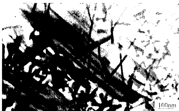
Fig. 1. Closely packed blocks of the same crystalline orientation nanowhiskers of \text{WO}_3 .
