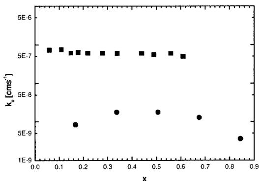
**Figure 3** Heterogeneous rate constant of the lithium insertion into high temperature prepared (circles) and solvothermally prepared Li<sub>4</sub>Ti<sub>5</sub>O<sub>12</sub> spinel
