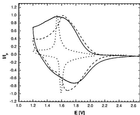
**Figure 2** Cyclic voltammograms of Li insertion into solvothermally prepared Li-Ti-O spinel annealed at 0, 200 and 300 °C. The material was prepared by reaction at 200 °C in water.
