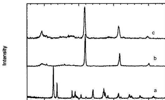
**Figure 1** X-ray diffraction patterns of: a) the starting  $\text{TiO}_2$  (mixture of rutile and anatase 1:3), b) product of the reaction in water, c) product of the reaction in ethanol. In both cases the reaction proceeded at 200 ° for 24 hours.
