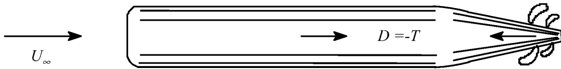
Figure 2. Free-Body Diagram for Undersea Vehicle Drag Analysis
