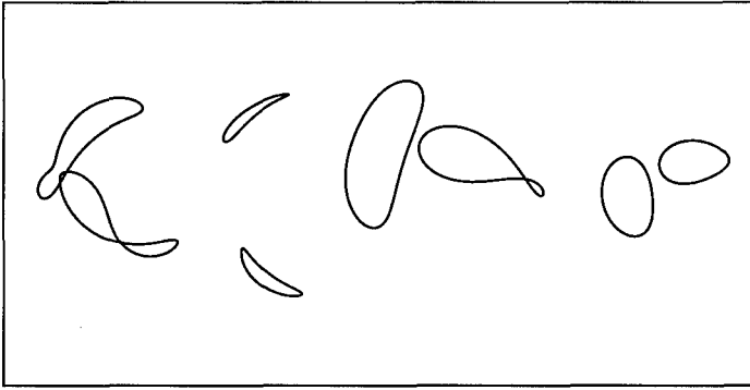
Fig. 8. Coupler curves for various values of the parameters k , r , R , a , b , c .
