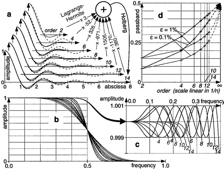
Fig. 5. Impulse responses of  $C^1$ -differentiable and 0.1%-precise Holberg interpolators (a) (Lagrange-Hermite in grey, *sinc* in dotted lines). Their Fourier transform (b) and an enlargement of them (c). The passband-*vs*-order diagram (d) showing the linear behaviour of Holberg interpolators and the parabolic behaviour of the Lagrange-Hermite interpolators.
