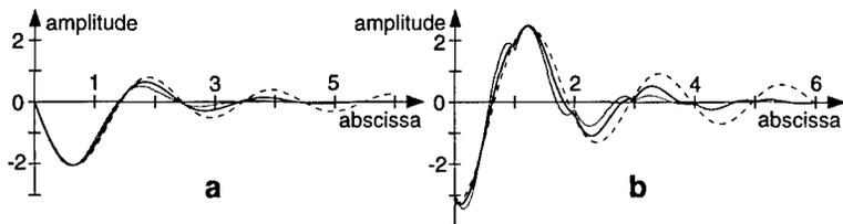
**Fig. 6.** Right part of the impulse responses of the 10th-order Lagrange-Hermite (in grey) and Holberg interpolators of first (a) and second (b) derivatives. Perfect (but truncated) interpolators for derivatives are displayed in dotted lines.
