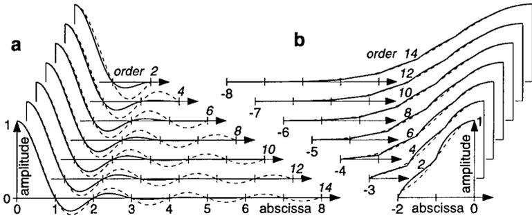
Fig. 4. Right part of the impulse responses of  $C^1$ -differentiable Lagrange-Hermite interpolators (a), sinc in dotted lines. Their left part divided by the sinc (b), as compared to Gaussian curves  $\exp(-\frac{x^2}{n+1/2})$ , in dotted lines.
