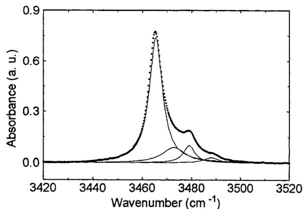
Figure 3. Decomposition of the  $\text{OH}^-$  stretching vibrational band in a nearly stoichiometric  $\text{LiNbO}_3$  crystal. Dots represent the experimental spectrum, continuous lines are the fitted Lorentzian components.
