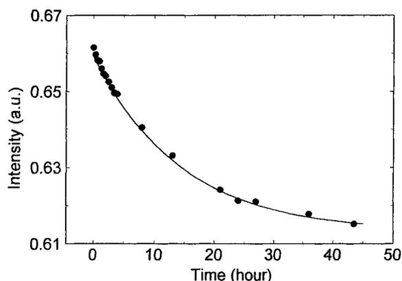
Figure 4. Intensity of the  $3465\text{ cm}^{-1}$   $\text{OH}^-$  band component as a function of time at  $110\text{ }^\circ\text{C}$ . An exponential decay curve (continuous line) was fitted to the experimental points (dots) resulting in a time constant of about 14.4 hours.
