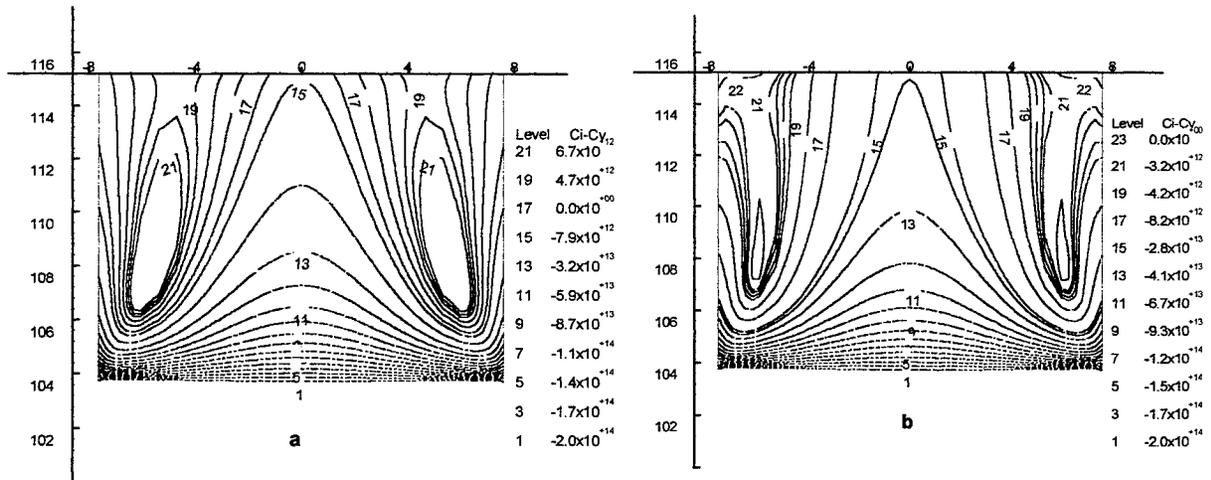
Fig.4. Isolines of the IPD concentration difference for the 50%-s growing stage and pull rates according to the mixed ( $v-i$ ) and vacancy ( $v$ ) growth modes: a -  $V_p = 0.42$  mm/min; b -  $0.47$  mm/min.
