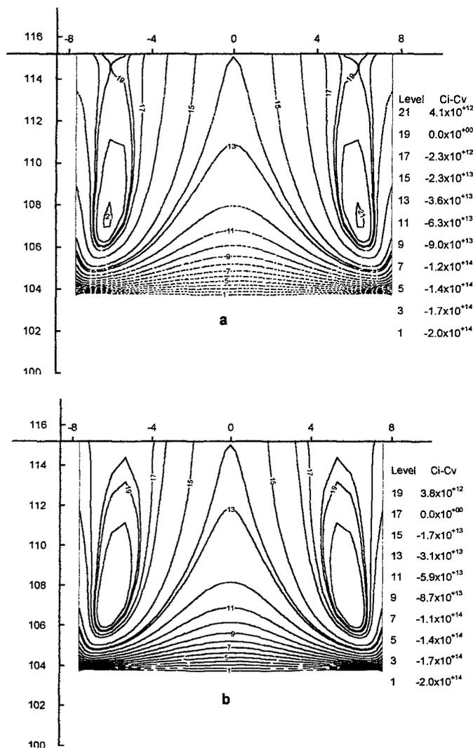
Fig.5. Isolines of the IPD concentration difference for various crystal growth stages at  $V_p = 0.50$  mm/min corresponding to the following growth modes:
