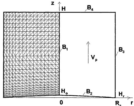
Fig. 2. Scheme of the calculation region (on the right) and according mesh of 6-nodes triangular finite elements (on the left). Here: B<sub>1</sub> - symmetry axis, B<sub>2</sub> - LSI, B<sub>3</sub> is crystal surface, B<sub>4</sub> is top boundary of a recombination.
