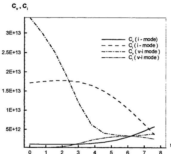
Fig.6. Radial distributions of  $C_v$  and  $C_i$  concentrations on the top boundary ( $z = H$ ) corresponding to pull rate variations at the 50%-s crystal growing stage. Here: the interstitial (i) mode is at  $V_p = 0.37$  mm/min, and the mixed (v-i) mode arises at  $V_p = 0.50$  mm/min.
