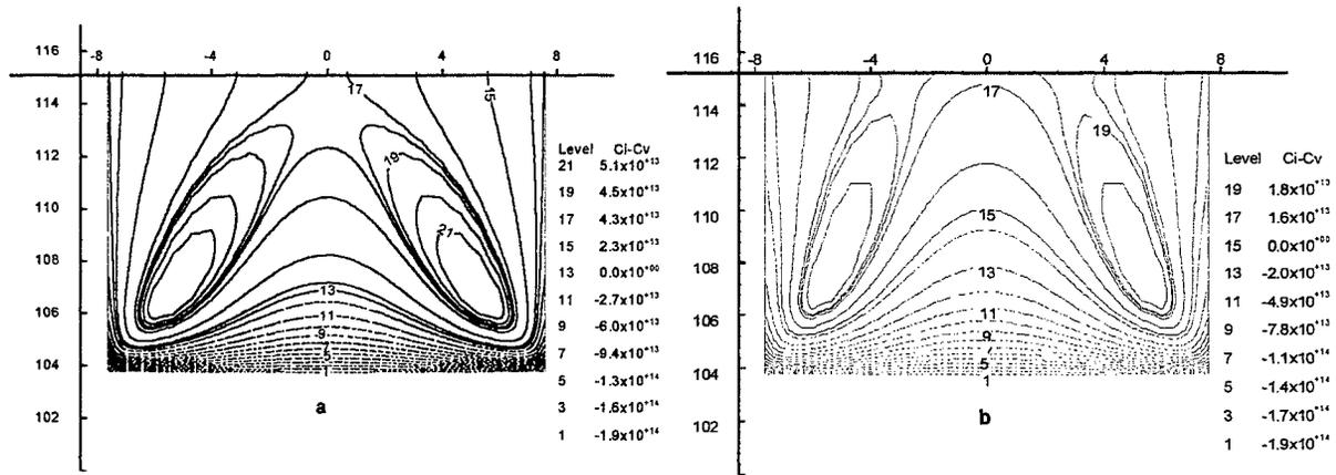
Fig.3. Isolines of the IPD concentration difference ( $C = C_i - C_v$  [ $\text{cm}^{-3}$ ]) for various crystal growth stages at the interstitial growth mode: a - 30% body,  $V_p = 0.39$  mm/min; b - 50%,  $V_p = 0.37$  mm/min.
