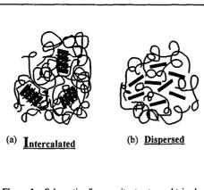
Figure 1. Schematic of composite structures obtained using layered silicates. The rectangular bars represent the silicate layers. (a) single polymer layers intercalated in the silicate galleries (intercalated); (b) composites obtained by delamination of the silicate particles and
