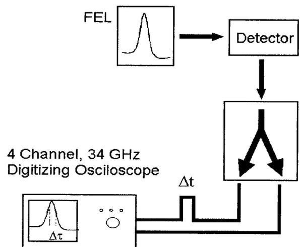
Fig. 1: Principal setup for the DEG method.
