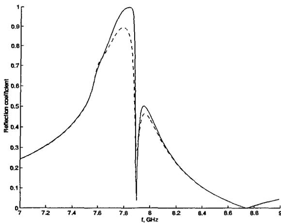
Figure 1: Reflection coefficient as function of frequency.
