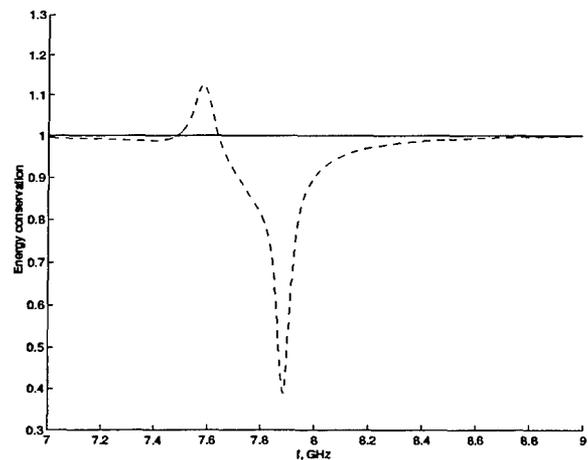
Figure 2: Energy conservation as function of frequency.
