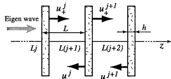
Figure 1: Infinite periodic layered structure of 2-D arrays
