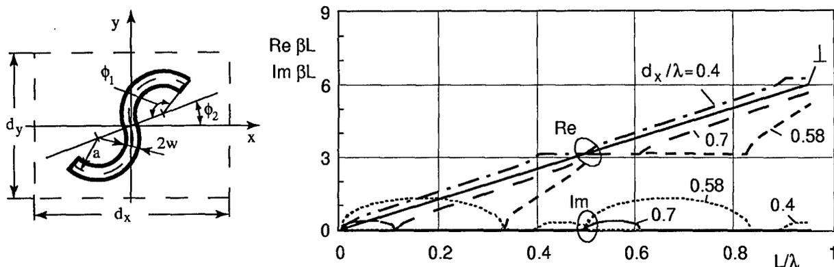
Figure 2: Propagation constant  $\beta$  versus distance between layers: array without substrate  $h = 0$ ,  $d_x = d_y = 10$  mm,  $a = 3$  mm,  $\phi_1 = \pi/2$ ,  $\phi_2 = 0$ ,  $w = 0.05$  mm,  $d_x/\lambda_0 \approx 0.58$  is resonant value.
