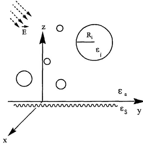
Figure 1 Geometry of the semi-infinite matrix disperse system.
