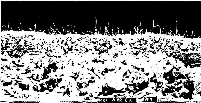
Fig.1 SEM micrographs show (a) as-grown bulk bundles, (b) multi-wall nanotubes embedded in bulk bundles, (c) cross-sectional image of screen-printed CNTs-emitters are perpendicular to substrate after surface treatment.
