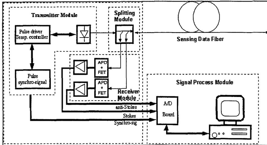
Fig. 5 Schematic of the DFTS experimental system
