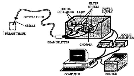
The two photo multiplier tubes convert the optical signal to the electrical signal, with the current being proportional to the optical signal intensity. The electrical signals are directed to the two lock-in amplifiers. A lock-in amplifier is a phase sensitive detector at a specific frequency, while rejecting all other signals. A personal computer is used to control the instrumentation, to process the amplified signals, and to display and store the ratio data.
