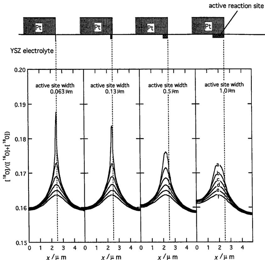
Fig. 4. Dependence of calculated isotope distribution on the active site width. The curves are isotope concentration profile in the depth of the electrolyte (a) 0  $\mu\text{m}$  (b) 0.031  $\mu\text{m}$ , (c) 0.063  $\mu\text{m}$ , (d) 0.09375  $\mu\text{m}$ , (e) 0.125  $\mu\text{m}$  and (f) 0.15625  $\mu\text{m}$ .
