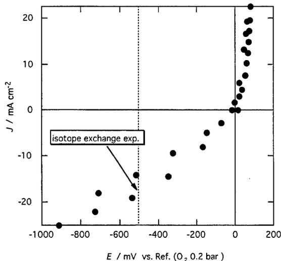
Fig. 8. Steady state polarization curve for Pt/YSZ sample at 973 K in 0.2 bar oxygen.
