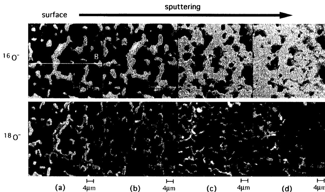
Fig. 9.  $^{16}\text{O}^-$  and  $^{18}\text{O}^-$  distribution in the sample treated at 973 K in 0.2 bar oxygen  $^{18}\text{O}$  under cathodic polarization ( $-0.5\text{ V}$ ) for 5 min. Images were taken at the surface (a); after sputtering 2 min. (b); 4 min. (c); and 6 min. (d).
