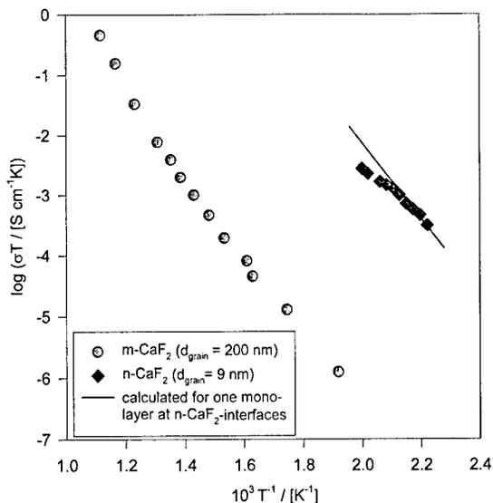
Fig. 3. Temperature dependence of the conductivities of nano- and micro-crystalline  $\text{CaF}_2$  derived from the high-frequency semicircles [5,9]. The line represents the estimated conductivities assuming a pronounced space charge effect [5].
