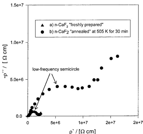
Fig. 2. Impedance spectra for nanocrystalline  $\text{CaF}_2$  samples (a) 'freshly prepared' and (b) 'annealed' [9].
