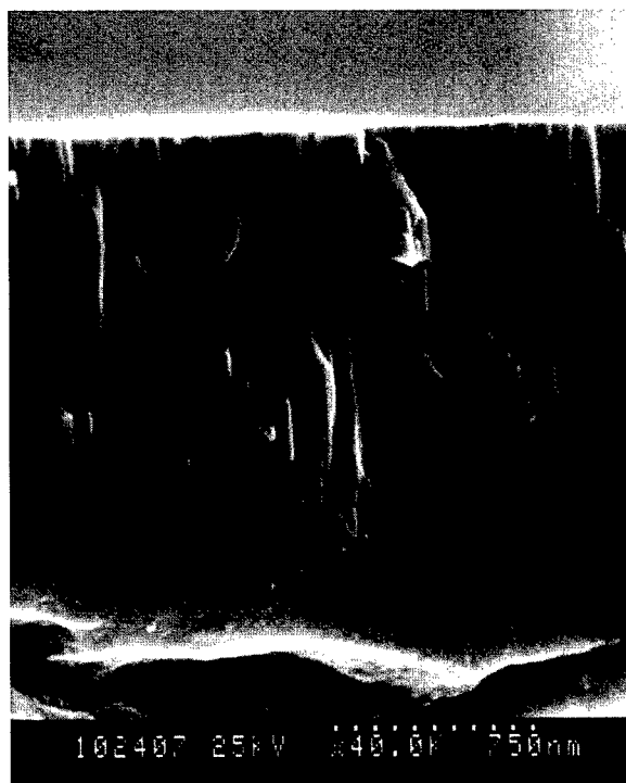
Fig. 6. SEM cross-sectional image of \delta - \text{Bi}_2\text{O}_3 electrodeposited onto a (111)-textured Au EQCM electrode. The image shows a high degree of columnar growth, typical of textured films. The thickness of the film as determined by SEM agrees well with that calculated from the EQCM. The bar marker is 750 nm.
