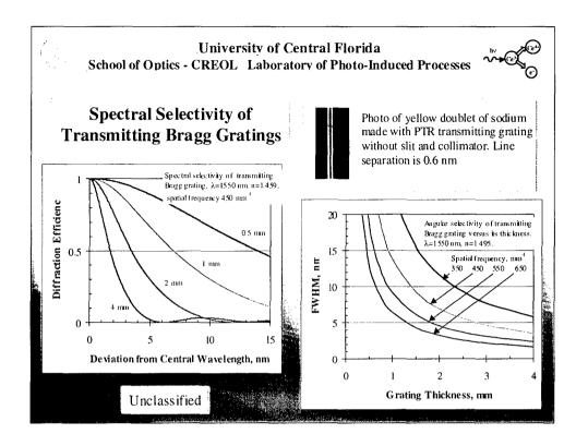
The spectral selectivity of Bragg gratings in PTR glass can be varied from parts of a nanometer to several tens of nanometers. One can see the photo of the sodium doublet with 0.6 nm separation between the lines. It should be noted that no slits and no collimators were used in making this photograph.
