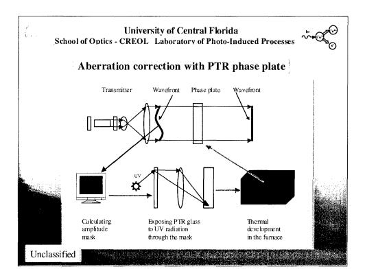
This illustrates how PTR glass can be used to correct aberrations or phase errors in an optical system. A mask is made of the aberration, and the conjugate of this is used to make the PTR glass phase plate. Insertion of the phase plate in the optical train will then correct for the aberration enabling "eagle-eye" vision to be built into the system.
