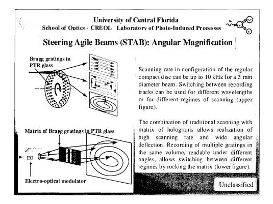
The use of a matrix of PTR Bragg gratings enables scanning the laser beam at arbitrary angles. This approach can be used as the sole one (upper scheme) or in combination with conventional electro-optical devices (lower scheme).
