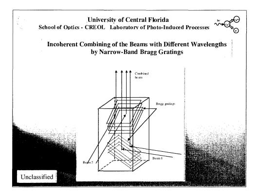
This figure illustrates how PTR glass should enable a designer to combine two beams from two different lasers into one beam. This is called incoherent beam combining. Coherent combining should also be achieved with this technology.CREOL currently has an effort sponsored by AFOSR and AFRL/DE to demonstrate incoherent beam combining of two 100W cw lasers in the manner shown in this viewgraph.
