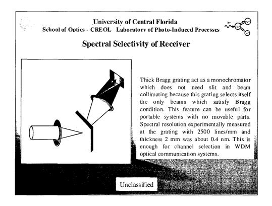
Spectral selection of a target can be achieved by the use of PTR glass. A resolution of 0.4 nm can be attained with a 2 mm thick grating. No monochromator with slits and collimators are needed. A portable spectrometer for selected wavelengths with subnanometer spectral resolution with no moving parts looks very promising. Recording of multiple gratings in the same volume allows detection of several spectral lines without tuning.
