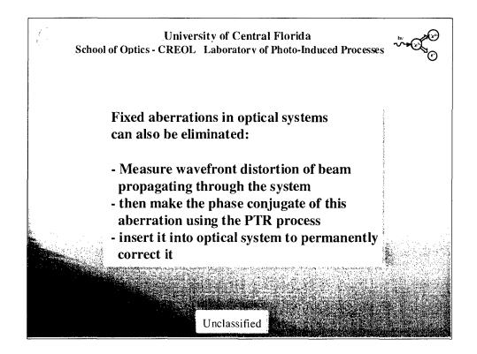
The third major application of PTR glass is for correction of fixed aberrations or phase nonuniformities in optical systems. This technology should enable an optical system manufacturer to correct the fixed errors in his optical system as a final step in the system manufacturing process. Such optical systems include telescopes, cameras, imaging systems, and the Hubble telescope.
