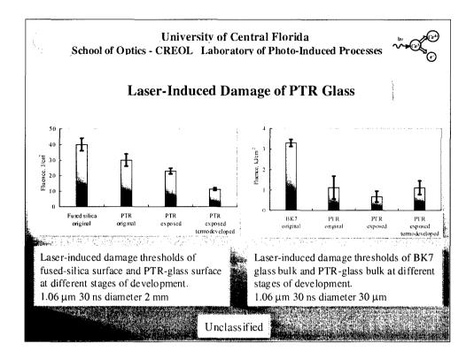
The laser-induced damage threshold of PTR glass was measured at the University of Rochester's Laboratory for Laser Energetics. It was found that exposed and developed PTR glass has a damage threshold for a 30 ns pulse of about 15 J/cm². This value is about 30 % of that for the best fused silica used at the Omega facility. So, PTR diffractive components can be used in high-peak-power laser systems.
