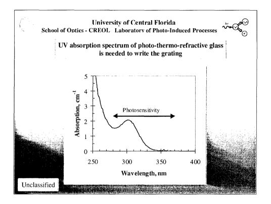
The UV absorption spectra of PTR glass is presented in this figure. The absorption band of Ce<sup>3+</sup> having a maximum at 305 nm is clearly seen. Photoionization of Ce<sup>3+</sup> triggers the chain of photoinduced processes in PTR glass resulting in precipitation of NaF microcrystals. It is important to note that NaF is a high-bandgap dielectric material that has no absorption in the UV, visible, and near-to-mid IR regions
