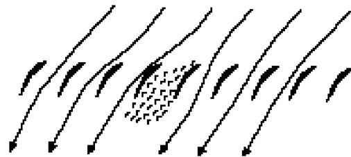
Figure 5 - Sketch of short-length scale rotating stall event. From Day [25].
