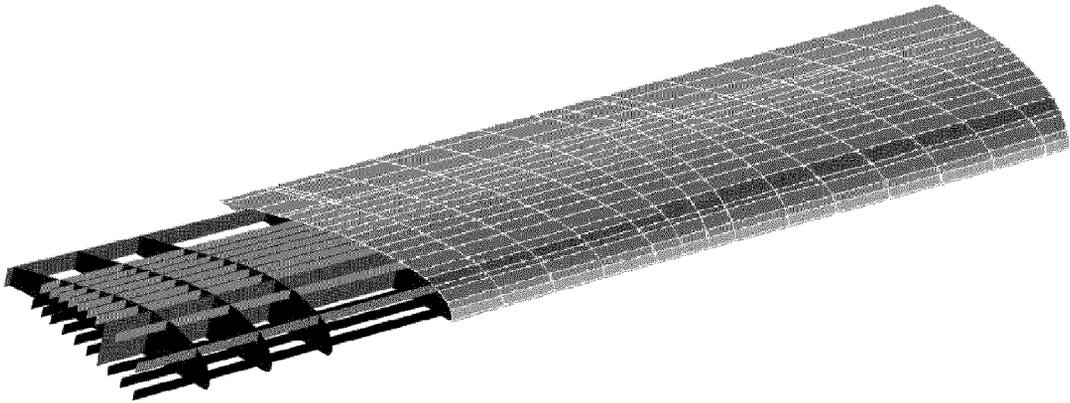
*Figure 5: Finite element model of the fowler flap*
