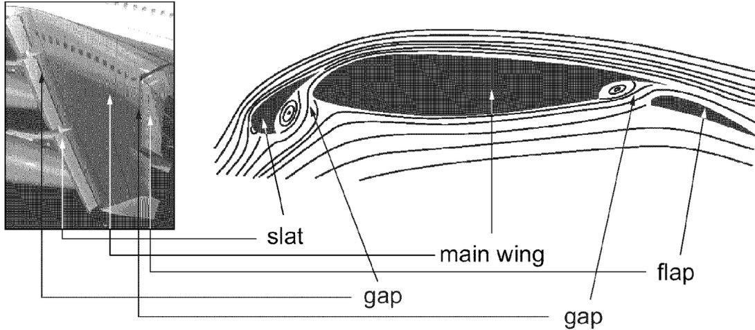
Figure 1: Airfoil with extended slat and flap
