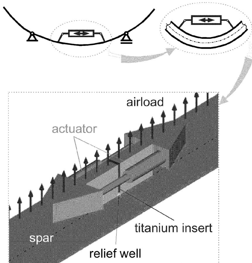
Figure 4: Integration of the actuator into the spar
