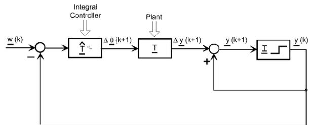
Fig. 13 Quasi-Steady Operating Closed Loop System
