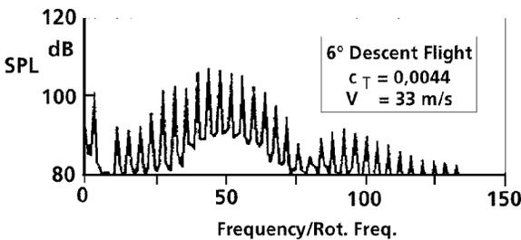
Fig. 8 Frequency Content of Rotor Noise
