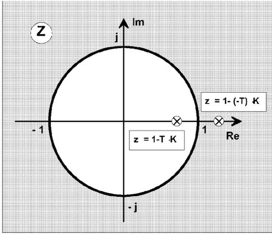
Fig. 16 Pole Placement for Conversion of Control Efficiency
