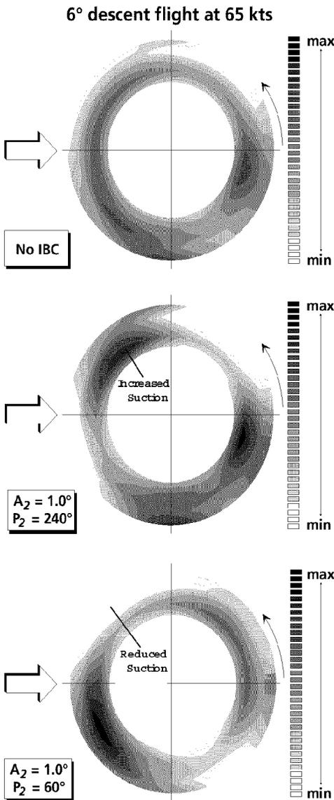
Fig. 4 Low Pass Filtered Leading Edge Pressure
