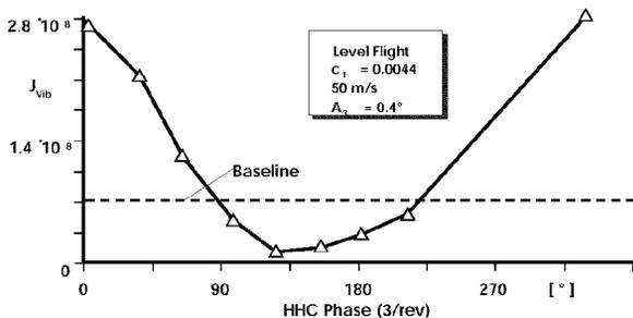
Fig. 14 Variation of Vibration Intrusion Index with 3/rev Phase Shift
