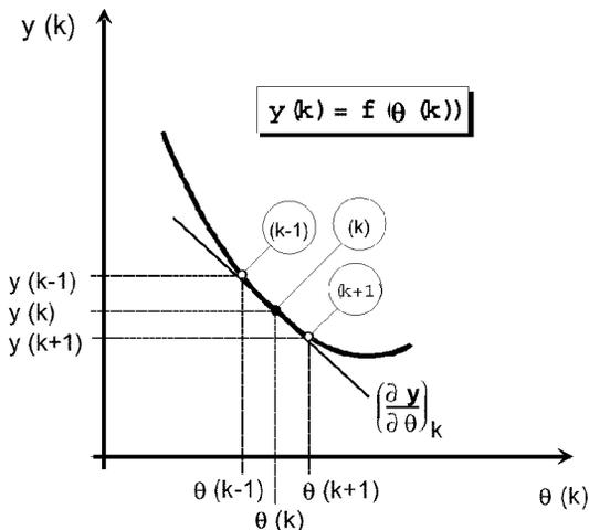
Fig. 12 Linearization Around Actual Point of Operation
