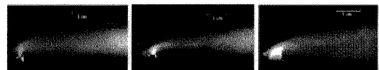
figure 14 Average side view for the CJ penetration (from left to right: CJ type rect1 , rect2 and circ )
