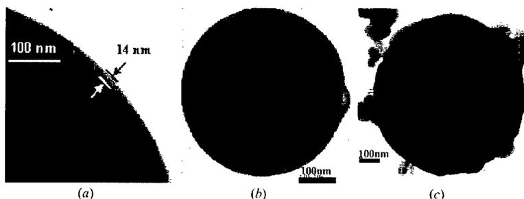
**Figure 7.** TEM micrographs of silica particles coated with (a)ethylene plasma polymer at 20W, 100 mTorr, and 1:1 Ar:ethylene flow rate; (b)styrene plasma polymer at 15W, 28 mTorr, and no Ar flow; (c)styrene plasma polymer at 15W, 470 mTorr, and 6:1 Ar:styrene flow rate.
