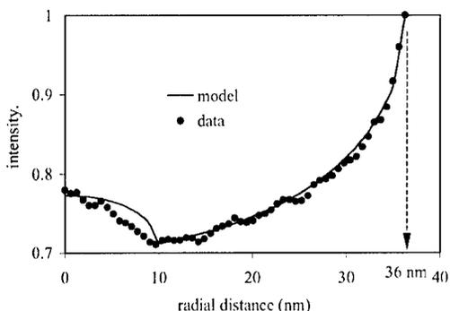
**Figure 4.** Radial intensity profile of a hollow styrene plasma polymer particle (intensity normalized to background). The particle radius is 36 nm with a core radius of 10 nm. The Beer-Bouguer model assumes an empty core but constant absorption coefficients.
