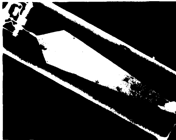
Figure 7. X-ray radiograph shows areas of corrosion.
