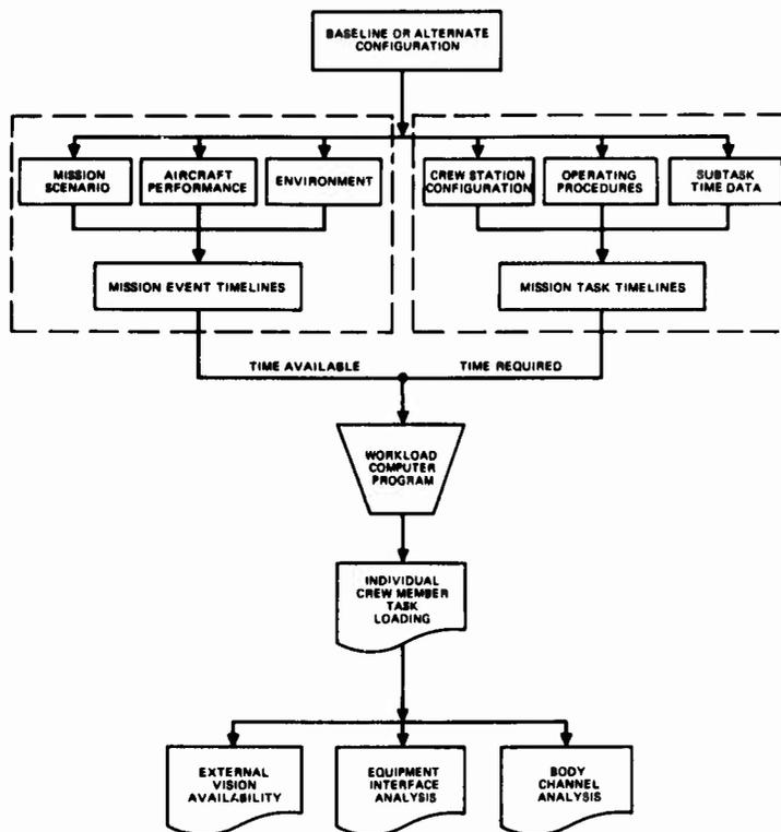
FIGURE 1. CREW STATION WORKLOAD ANALYSIS AND DESIGN SYSTEM (CWADS)
