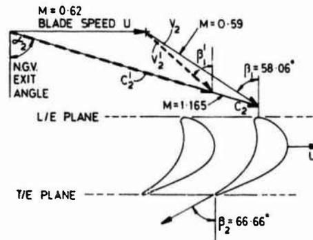
Fig. 1(b) Velocity triangles at inlet for the steady nominal design case at mid-span, showing the reduced incidence caused by the deficit in the wake.
