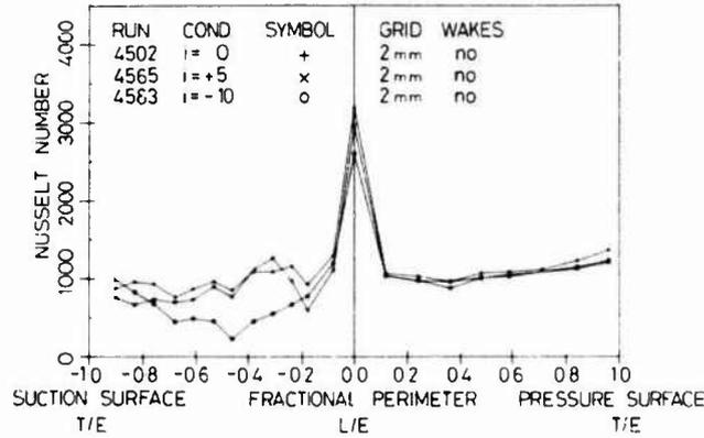
Fig. 4(a) Effect of incidence variation on mean heat transfer rates at the nominal design case ( $M_2 = 1.18$ ,  $Re = 0.919E6$ ) with no wake and shock interaction.
