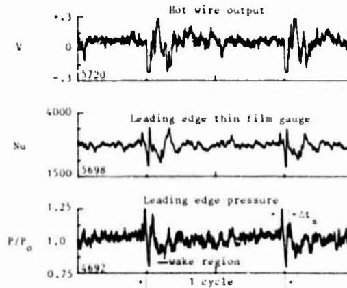
Fig. 5(b) Measurements of the unsteady disturbance at inlet by a hot-wire in the freestream and heat transfer and pressure measurements at the stagnation point.
