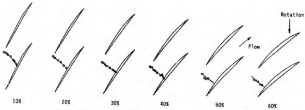
Figure 5. - Shock location in blade-to-blade plane for six spanwise locations at Peak Efficiency Flow Rate.
