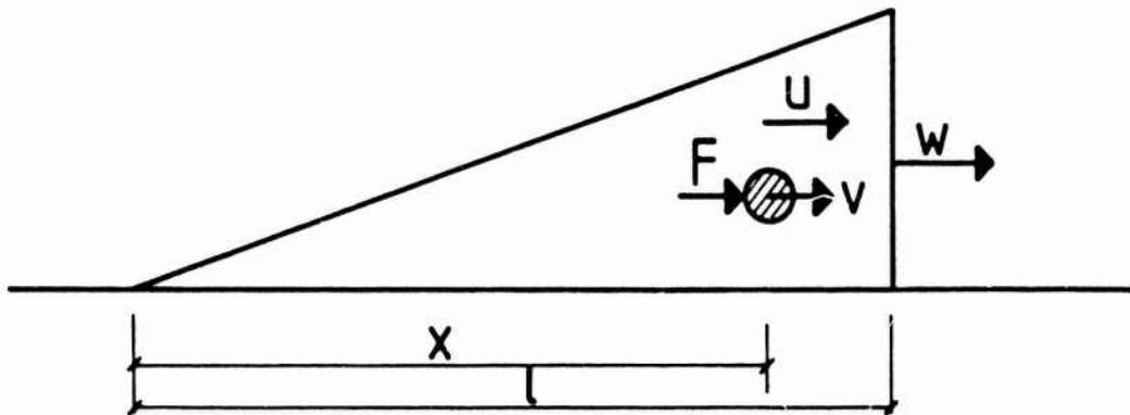
Figure 3. Simplified model for calculation of debris velocity.
