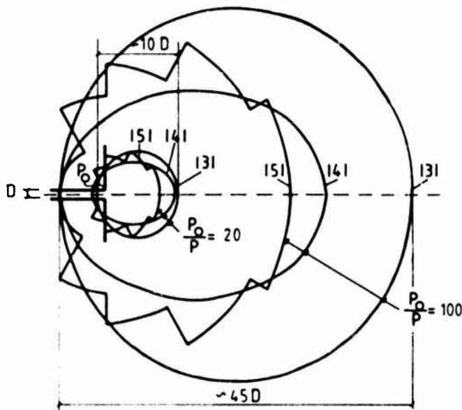
Figure 1. Comparison of different formulas for the overpressure outside a tunnel entrance from /3/, /4/ and /5/.
