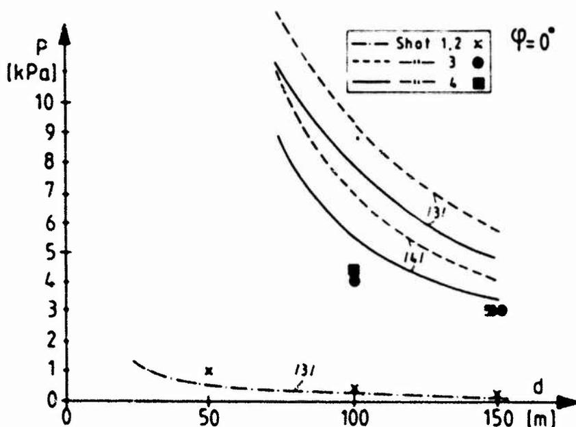
Figure 8. Measured overpressure outside the tunnel entrance
